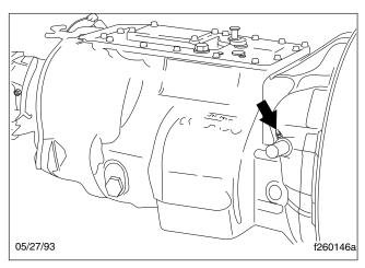
Fig. 4, Cross-Shaft Grease Fitting, Right Side
