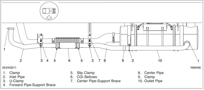
Fig. 6, CAT EPA07 Exhaust Installation with CGI Bellows
