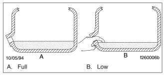
Fig. 8, Mercedes-Benz Transmission Fluid Level Checking
