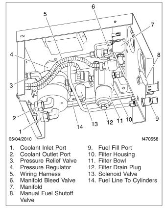
Fig. 11, CNG Fuel Panel Components
