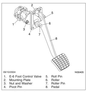
Fig. 9, Brake Pedal and Valve Assembly
