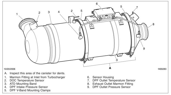
Fig. 4, Typical Aftertreatment Device
