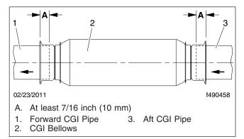
Fig. 9, CGI Bellows Installation
