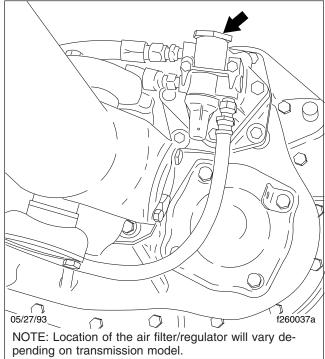
Fig. 4, Eaton Fuller Transmission Air Filter/Regulator Location
