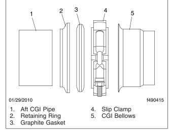
Fig. 8, Aft Facing Slip Clamp Installation
