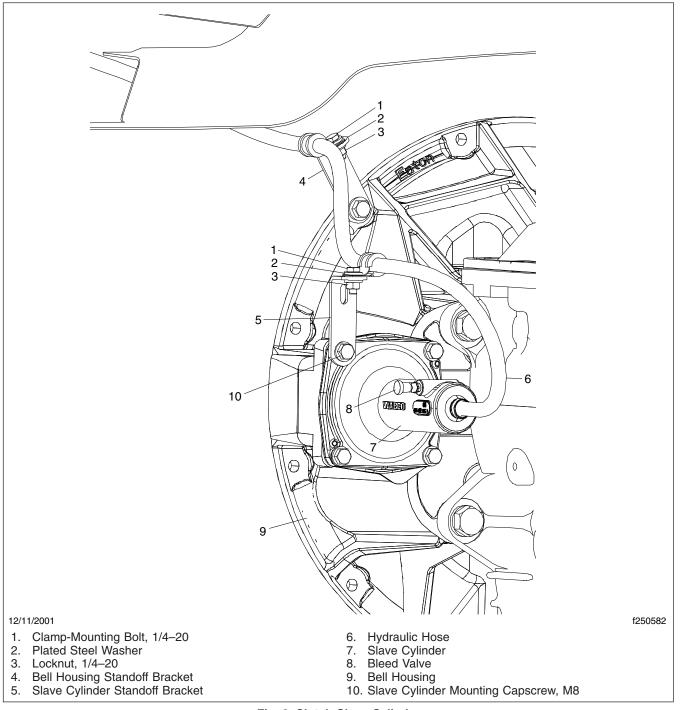
Fig. 6, Clutch Slave Cylinder
