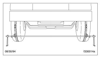
Fig. 10, Trammel Bar Positioning
