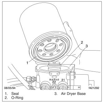
Fig. 11, Desiccant Cartridge Replacement
