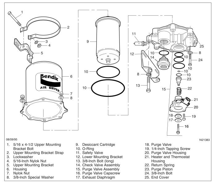
Fig. 1, AD-9 Air Dryer (exploded view)
