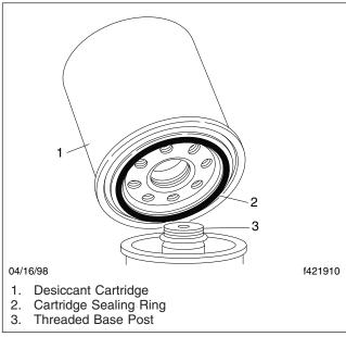
Fig. 3, Desiccant Cartridge Replacement
