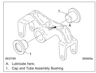
Fig. 8, Equalizer Assembly Lubrication
