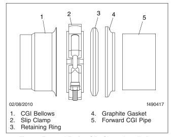
Fig. 10, Forward Facing Slip Clamp Installation
