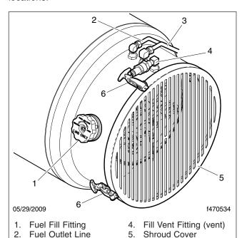
Fig. 4, Fuel Tank Outer Shell
