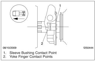
Fig. 2, Grease the Contact Points
