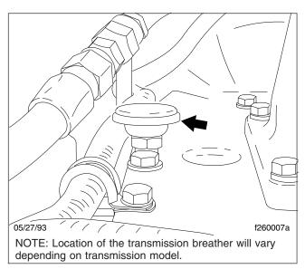
Fig. 3, Transmission Breather (Eaton Fuller shown)
