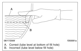
Fig. 1, Axle Lubricant Level Inspection
