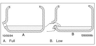
Fig. 1, Transmission Oil Level Checking
