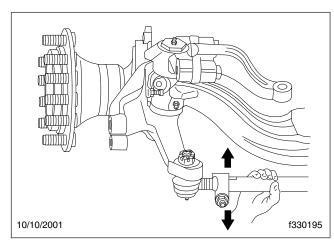
Fig. 7, Check Movement of Tie Rod End
