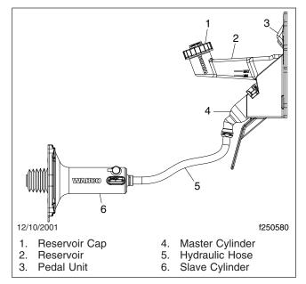
Fig. 5, Clutch Components
