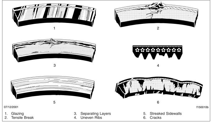
Fig. 1, Drive Belt Replacement Conditions
