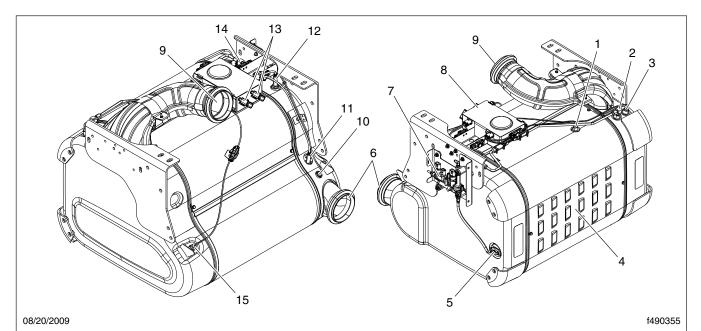
NOTE: The sensor box (item 8) contains the SCR inlet and outlet NOx sensors, DPF outlet pressure sensor, and the DOC inlet pressure sensor.
