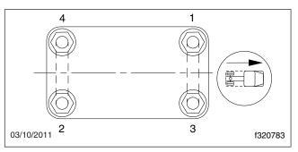
Fig. 9, Tightening Pattern for U-Bolt High Nuts
