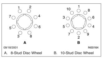
Fig. 1, Wheel Nut Tightening Sequence
