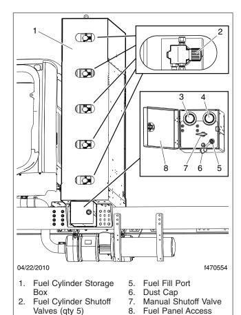
Fig. 9, CNG Fuel Cylinder Storage Box (5-cylinder system shown)
