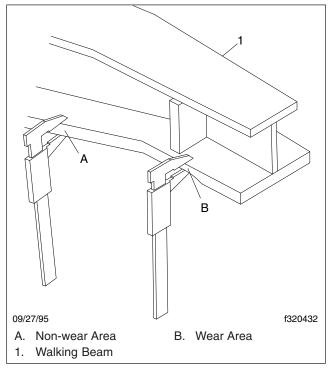
Fig. 7, Walking Beam End Wear Thickness
