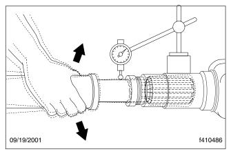
Fig. 3, Examine the Slip Yoke Spline
