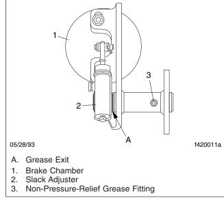
Fig. 7, Camshaft Bracket Lubrication
