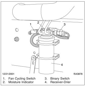
Fig. 1, Receiver-Drier
