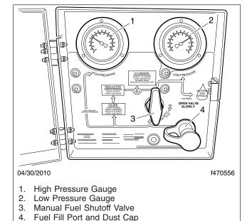
Fig. 8, CNG Fuel Panel
