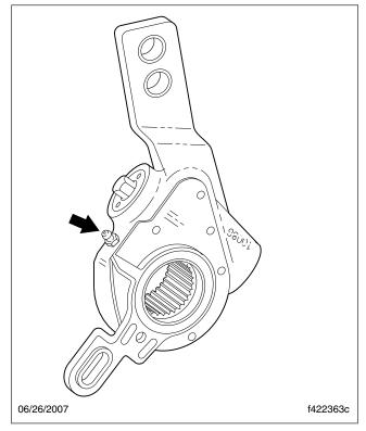
Fig. 5, Haldex Automatic Slack Adjuster Grease Fitting
