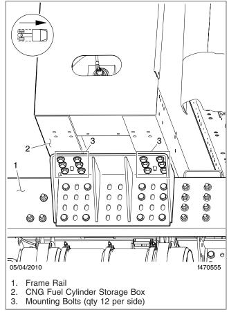
Fig. 7, Fuel Cylinder Storage Box Mounting Bracket (passenger side shown)
