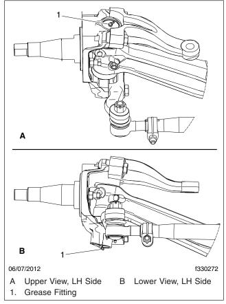
Fig. 1, Grease Fittings, Detroit Axles
