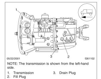
Fig. 7, Mercedes-Benz Transmission Drain and Fill Plugs
