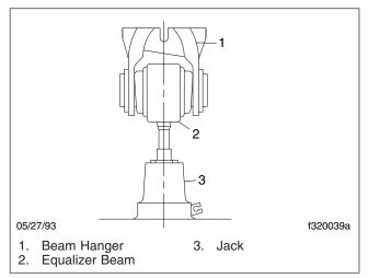
Fig. 4, Raising the Beam End
