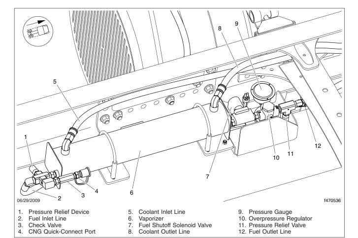
Fig. 6, LNG Vaporizer Assembly
