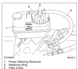
Fig. 1, Power Steering Reservoir
