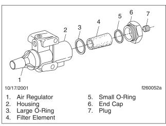
Fig. 5, Eaton Fuller Transmission Air Filter/Regulator Components
