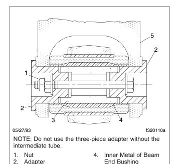
Fig. 5, Three-Piece Adapter-Type Beam End Connection
