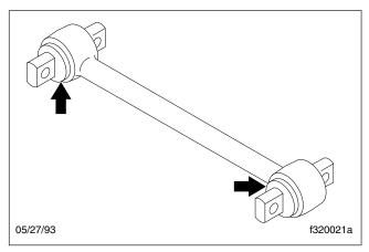
Fig. 1, Torque Arm Bushings
