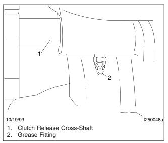
Fig. 3, Cross-Shaft Grease Fitting, Left Side
