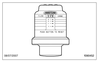
Fig. 1, Manual-Reset Air Restriction Indicator, Graduated
