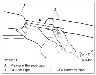
Fig. 7, Measuring the Pipe Gap (typical)
