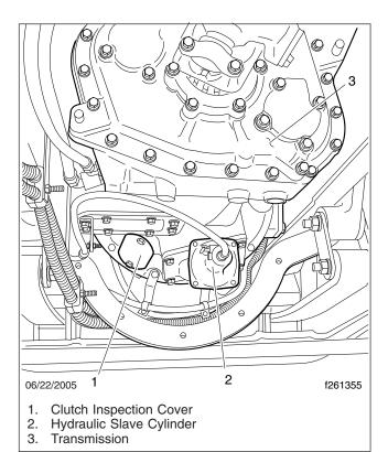
Fig. 8, View from Underneath the Vehicle
