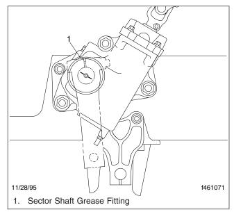
Fig. 2, Steering Gear Lubrication
