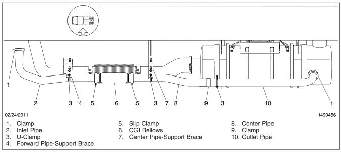
Fig. 5, CAT EPA07 Exhaust Installation with CGI Bellows
