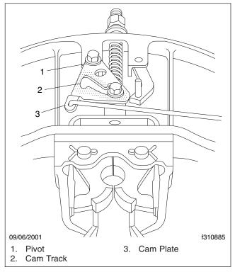
Fig. 7, Holland Fifth Wheel Cam Plate
