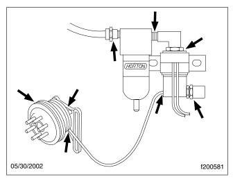
Fig. 1, Checking for Air Leaks (Horton DriveMaster)
