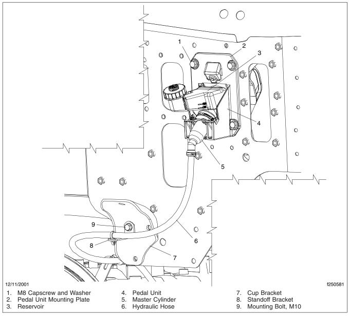
Fig. 7, Clutch Master Cylinder
