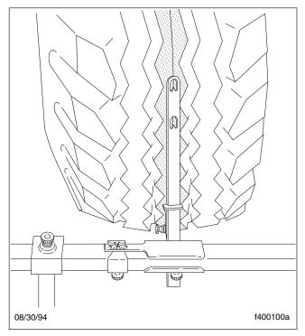
Fig. 11, Setting Trammel Bar Pointers
