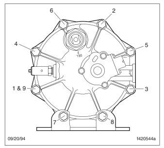
Fig. 2, AD-9 End Cover to Housing Torque Pattern
