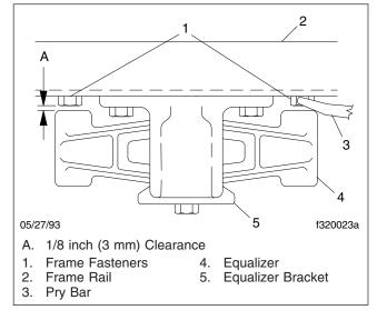
Fig. 3, Top View of the Equalizer
