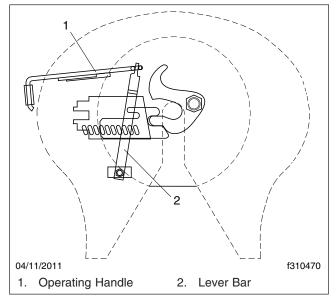
Fig. 2, Lever Bar and Operating Handle Alignment
