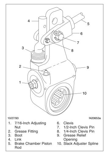
Fig. 6, Gunite Automatic Slack Adjuster
