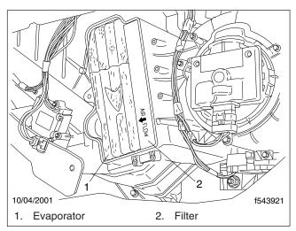
Fig. 2, HVAC Assembly Filter
