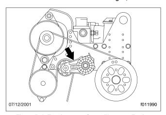
Fig. 2, Belt Tensioner on Caterpillar 3126 Engine
