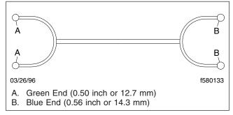
Fig. 9, Release Bearing Travel Tool A02-12419-000
