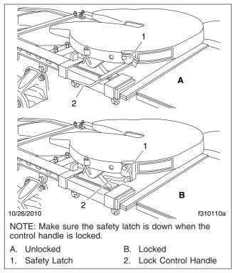
Fig. 10.2, Fontaine Locking Mechanism
