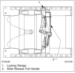
Fig. 10.11, Manual Release Sliding Fifth Wheel (Fontaine shown)
