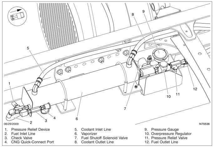
Fig. 11.10, LNG Vaporizer Assembly
