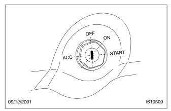
Fig. 16.10, Ignition Switch Positions
