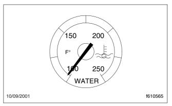
Fig. 3.9, Coolant Temperature Gauge
