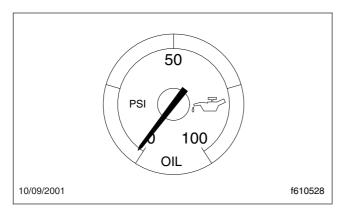
Fig. 3.10, Engine Oil Pressure Gauge
