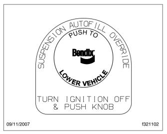
Fig. 4.34, Suspension Autofill Override Valve
