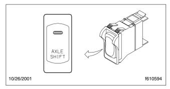
Fig. 8.24, Axle Shift Switch
