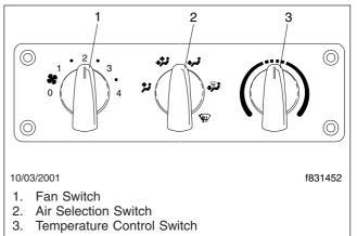
Fig. 4.35, HVAC Climate Control Panel, Standard
