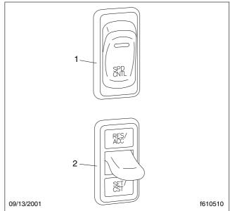
To turn cruise control on, press the upper half of the On/Off (rocker) switch. To turn cruise control off, press the lower half of the On/Off (rocker) switch.
