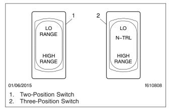
Fig. 4.28, Transfer Case Range Switches
