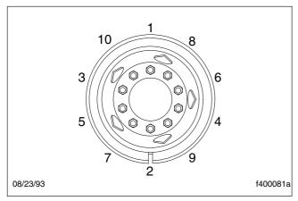
Fig. 11.4, Tightening Pattern, 10-Hole Wheels
