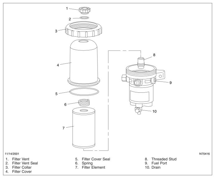
Fig. 13.2, Davco Model 232 and 233 Fuel/Water Separator
