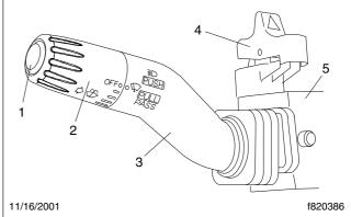
Press down on the upper part of the rocker to activate the hazard warning flashers.
