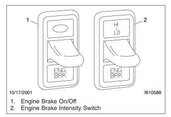
Fig. 7.17, Engine Brake Switches
