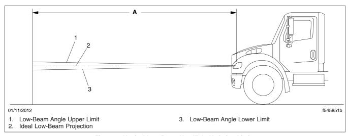
Fig. 14.3, Vertical Low-Beam Headlight Variation Limits
