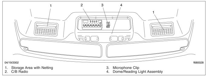
Fig. 3.16, Overhead Instrument Panel
