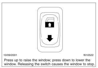
Fig. 5.1, Power Window Switch
