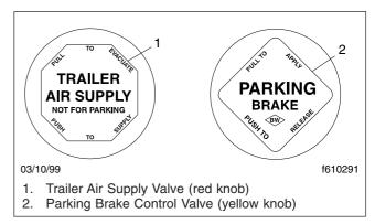
Fig. 4.29, Brake Valve Control Knobs
