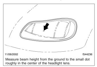
Fig. 14.1, Headlight Beam Height Adjusting Dot
