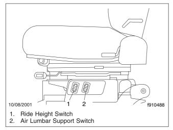
Fig. 5.16, Air Controls, Sears Seat
