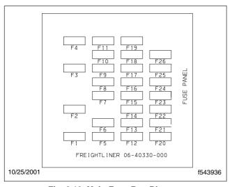
Fig. 2.12, Main Fuse Box Diagram
