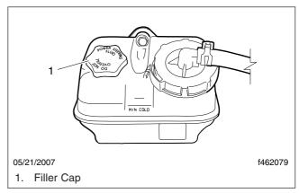
Fig. 11.6, Power Steering Fluid Reservoir
