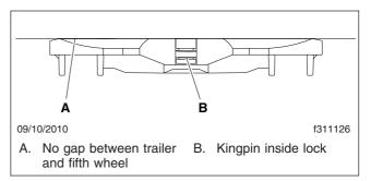
Fig. 10.6, Coupling Inspection
