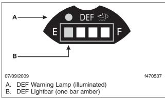
Fig. 7.11, DEF Level Low Initial Warning
