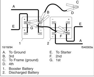
Fig. 13.5, Jumper Connections
