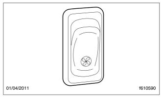
Fig. 4.21, Engine Fan Switch
