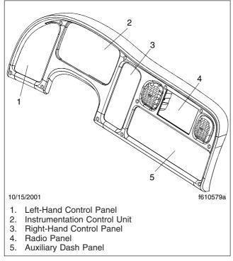
Fig. 4.2, Switch and Gauge Panels
