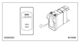
Fig. 8.21, Differential Lock Switch
