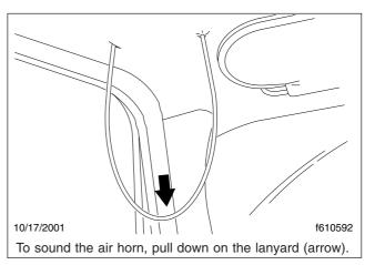
Fig. 4.15, Air Horn Control
