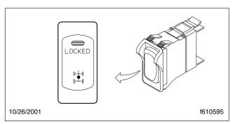
Fig. 4.25, Interaxle Lock Switch
