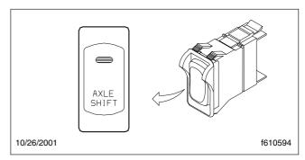
Fig. 4.26, Axle Shift Switch
