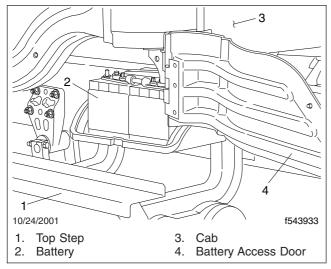
Fig. 13.4, Battery Compartment, Open
