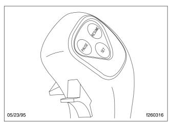
Fig. 7.16, Cruise Control Buttons on the Transmission Shift Knob
