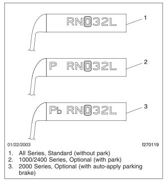
Fig. 4.22, Steering Column-Mounted Shift Controls
