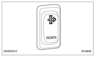
Fig. 4.16, Request/Inhibit Regen Switch
