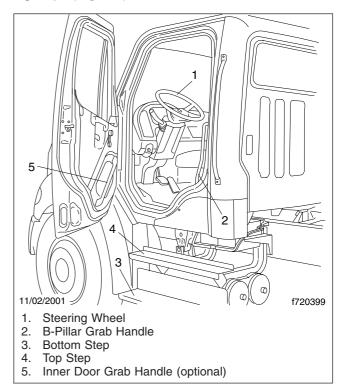
Fig. 2.4, Cab Access System, Driver's Side
