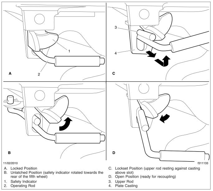
Fig. 10.9, Holland Kingpin Locking Mechanism
