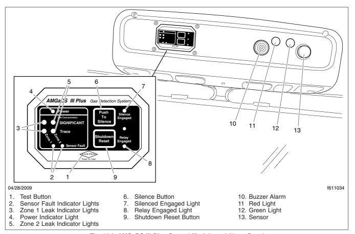
Fig. 16.9, AMGaDS III Plus Control Module and Alarm Panel
