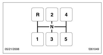
Fig. 8.3, Shift Pattern, 5-Speed FS Models
