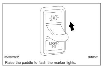
Fig. 4.5, Marker Light Interrupt Switch
