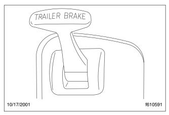
Fig. 4.30, Trailer Brake Lever
