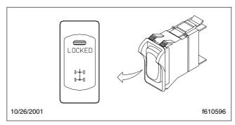
Fig. 4.24, Differential Lock Switch
