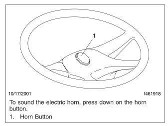
Fig. 4.14, Electric Horn Control
