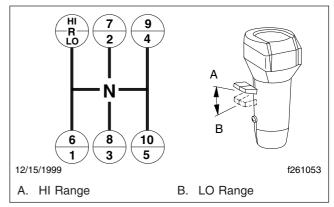
Fig. 8.7, Shift Pattern, 10-Speed Models
