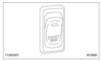
Fig. 7.18, Exhaust Brake Switch
