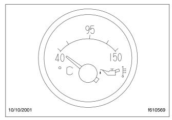
Fig. 3.11, Engine Oil Temperature Gauge
