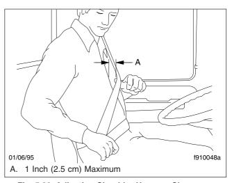
Fig. 5.20, Adjusting Shoulder Harness Clearance, Comfort Clip
