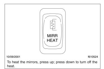
Fig. 5.3, Mirror Heat Switch
