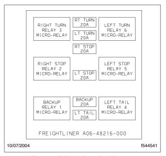
Fig. 2.14, Taillight Fuse Box Diagram
