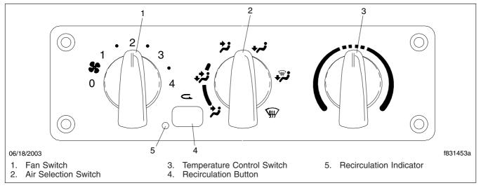
Fig. 6.2, Climate Control Panel With Air Conditioning
