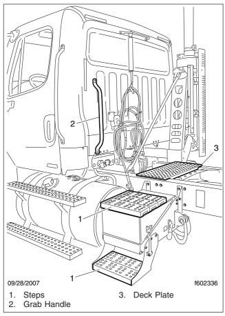
Fig. 2.6, Back-of-Cab Access Supports (typical)
