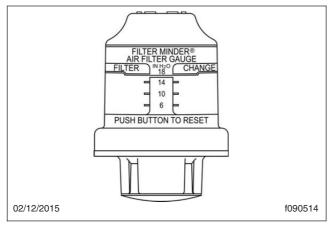
Fig. 3.6, Air Intake Restriction Indicator
