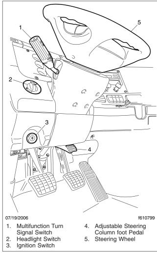
Fig. 4.32, Adjustable Steering Column
