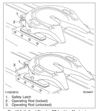
Fig. 10.3, Holland Simplex SE Locking Mechanism
