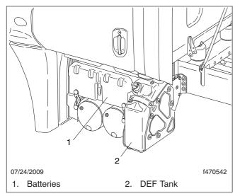
Fig. 7.8, DEF Tank Located Behind the Battery Box
