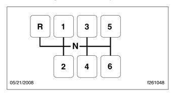
Fig. 8.4, Shift Pattern, 6-Speed FS and FSO Models
