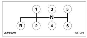
Fig. 8.19, Shift Pattern, M-B Transmissions
