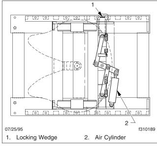
Fig. 10.15, Air-Operated Sliding Fifth Wheel (Fontaine shown)
