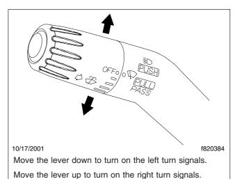
Fig. 4.11, Turn Signal Controls
