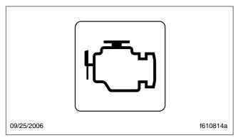
Fig. 7.5, Malfunction Indicator Lamp (MIL)
