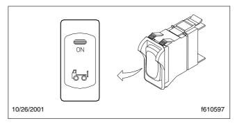
Fig. 4.33, Suspension Dump Switch
