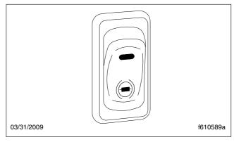
Fig. 7.19, Exhaust Brake Switch
