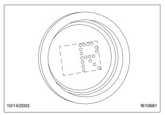
Fig. 8.17, Reverse Gear Display
