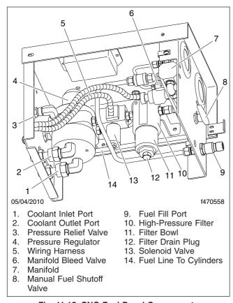
Fig. 11.15, CNG Fuel Panel Components
