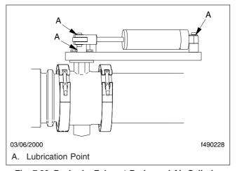
Fig. 7.20, Pacbrake Exhaust Brake and Air Cylinder
