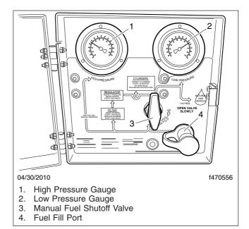
Fig. 11.9, CNG Fuel Panel
