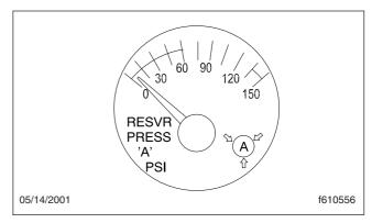
Fig. 3.14, Air Pressure Gauge (reservoir A shown)
