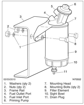
Fig. 11.11, Alliance Fuel/Water Separator Assembly and Installation
