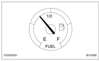
Fig. 3.12, Fuel Level Gauge, Pre-EPA10
