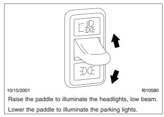
Fig. 4.3, Headlight/Parking Light Switch
